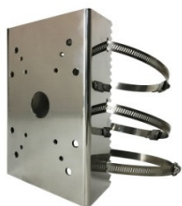
ON-PO01S / Pole Mount SUS316L, Poles 4 to 6" diameter 240 x 163 x 72mm, 1.6kgs
