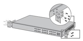
Put POE switch on the appropriate location of the rack, crutch by bracket; using the L-shaped bracket to fix the two sides of rack with screw, make sure POE switch is installed on the rack smooth and steady.
