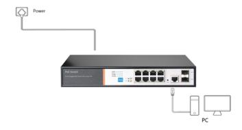
**Step 2.** Manually changed the computer IP address to 192.168.254.X (X is  $2 \sim 254$ ), subnet mask is 255.255.255.0
