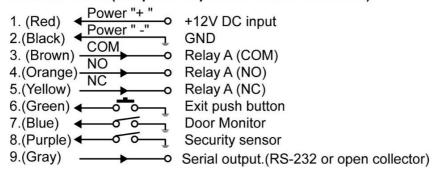
\*Once the 1100 (Disable the door monitoring function) parameter be set, the blue wire should be connected to GND.
