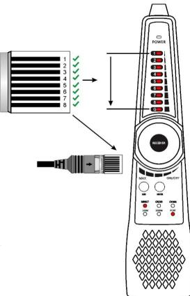
Press "MUTE" button, when the indicator light of port is on, the 1-8 and G indicator lights will show the connection of the line of the RJ45 connector or within 1 meter from RJ45 connector. As shown on the right, If the light is on, it means it is connected and vice versa.
