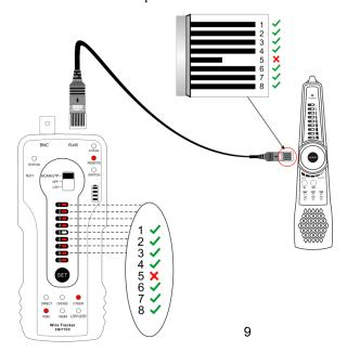
The middle of cable (mid-end) continuity detection: If the cable sequence detects that the pins of the cable are disconnected, and the local / remote pins are detected to be connected, indicating that the break point of the cable is in the middle position away from the ports on both sides.
