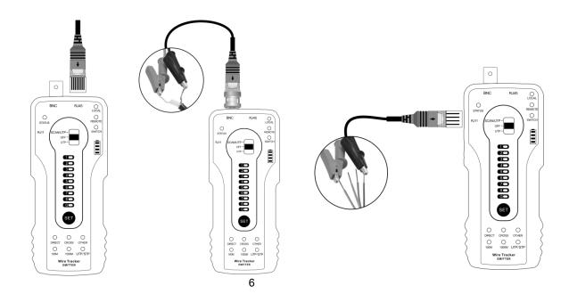
(1) Adjust the switch of emitter to the "Scan/UTP" mode, press "SET" key to switch to UTP/STP mode. The green light of the "UTP/STP" indicator means normal mode, while the red light is shielded mode. Turn on the wire receiver model at the same time to trace the wire.
