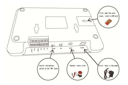
**Caution:** If you power on the host first and then insert the SIM card, the host possibly can not receive the signal or the circuit will be burnt. If GSM signal is normal, the power light will flash .
