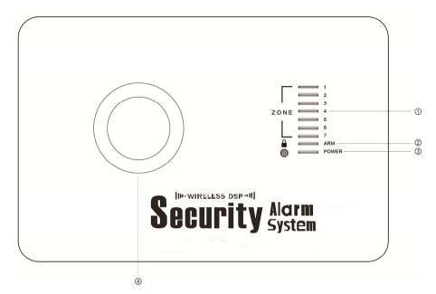
① Indicator light of defense zone: When alarming, the flashing indicator light means the corresponding defense zone is alarming.
