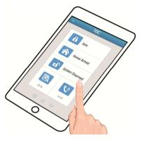
③Disarm by calling or texting remotely. Call the phone numbers of the host, input the operation password as voice prompt, and then press "2" Or texting the message "Operation Password XXXX" + "2" to the host.
