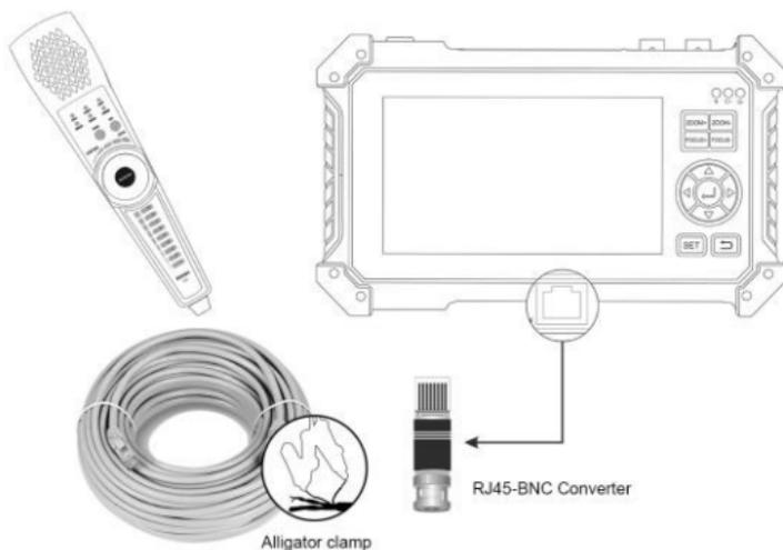
**Locate cables:** Arrow keys to switch mode, “UTP mode” to looking for unshielded network or telephone cables, “BNC mode” for finding BNC cable after connecting adapter. “STP mode” is used to find the shielded network cable. Turn on the cable tracer. The round knob, if clockwise rotation the knob to increase sensitivity, and turn it counter clockwise to decrease the sensitivity.
